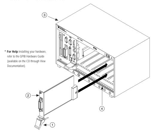
**C**. Screw the front panel of the PXI-GPIB to the chassis's injector/ejector rail.
